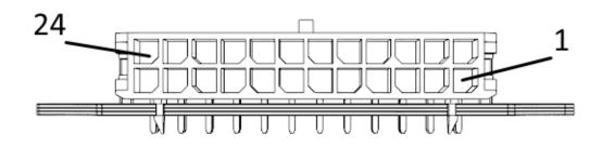
Converter has 12 contact pairs which are M-BUS interfaces. Converter provide connection up to 10 M-BUS devices. You can choose any 10 contact pairs. Wherein 1-2 contacts are M-BUS- (bot row), and 13-24 contacts are M-BUS+ (top row).
