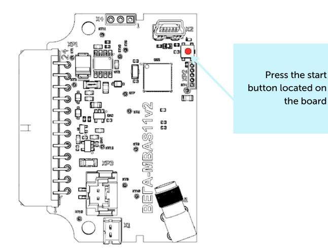
**2. OTAA.** After pressing the start button, the device makes three attempts to connect to the network within the set frequency plan. After the activation in the LoRaWAN network is confirmed, the device sends a signal (LED flashing for 5 seconds) and switches to the "Active" mode. If all attempts fail, the converter will continue to accumulate data and will attempt to connect to the network every 6 hours.
